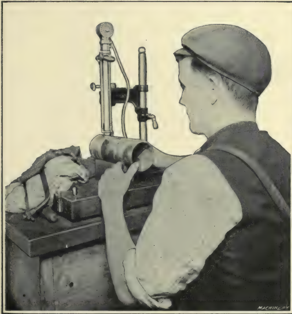
Fig. 10. Testing Hardness of Shrapnel Shells with Shore Scleroscope
